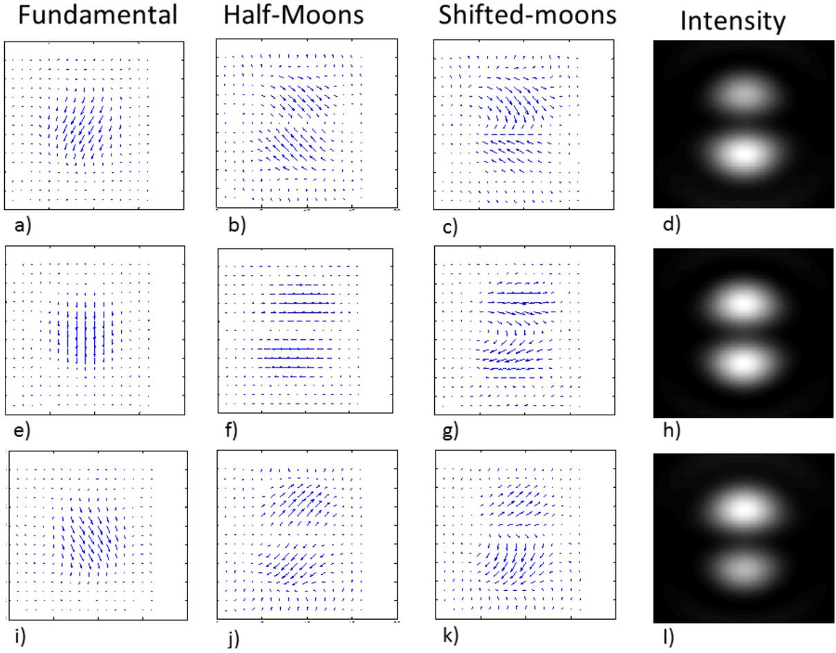
Figure 4. Simulation of patterns obtain at  $\rho_0=0.45$  before focal plane ( $Z=-0.2Z_{Airy}$  a) to d)), at focal plane ( $Z=0$ ; e) to h) ) and after focal plane ( $Z=0.2Z_{Airy}$  i) to l) ). The Shifted-Moons pattern (c,d,g,h,k,l) is the addition of a Half-Moon pattern (b f and j) and an Fundamental beam (a e and i).
