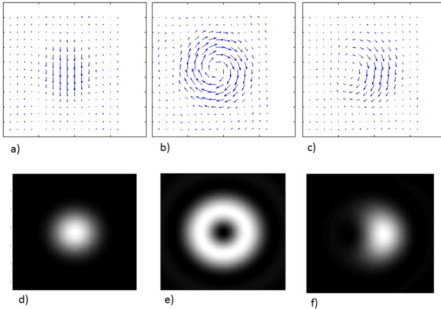
Figure 1. Representation of a fundamental beam a) and d) , a vortex beam b) and e), and the addition of the two beams c) and f).
