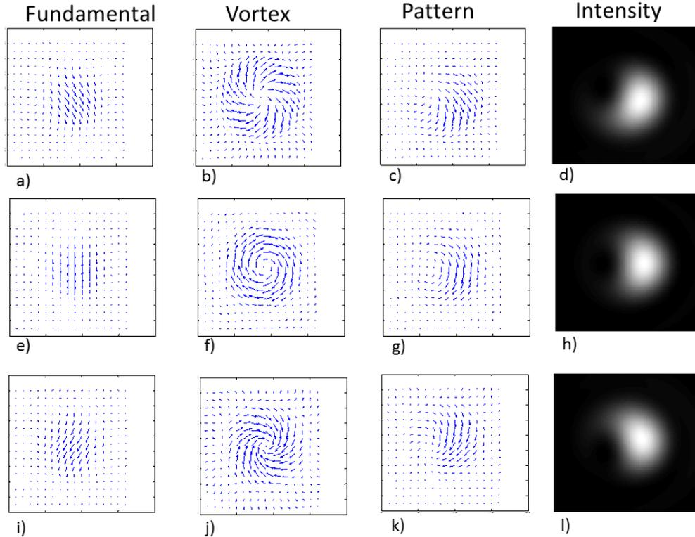
Figure 3. Simulation of patterns obtain at  $\rho_0=0.45$  before focal plane ( $Z=-0.2Z_{Airy}$  a) to d)), at focal plane ( $Z=0$ ; e) to h) ) and after focal plane ( $Z=0.2Z_{Airy}$  i) to l) ). The Stokes pattern (c,d,g,h,k,l) is the addition of a Vortex beam (b f and j) and an Fundamental beam (a e and i).
