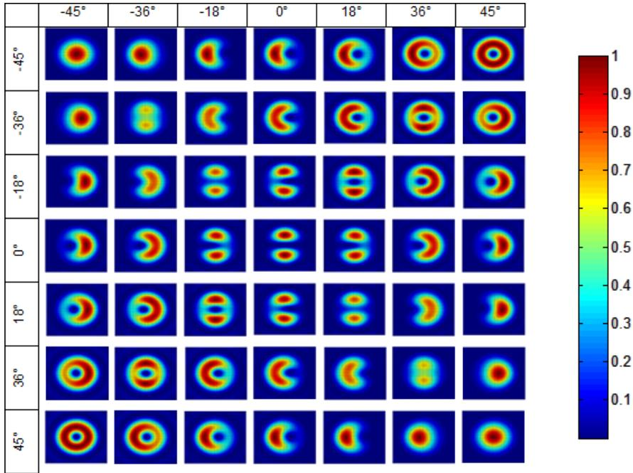
Figure 2. Table showing several patterns in the focal plane, obtained with elliptic polarizer with orthogonal orientations of their fast axis and varying ellipticity.
