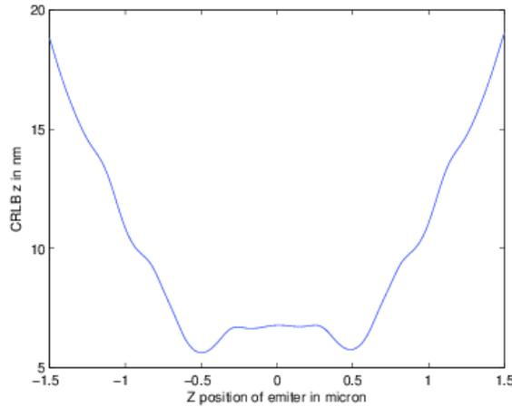
Figure 9.  $CRLB_z$  of a PSF shaped by astigmatism with parameter  $c_{AST}=20000$
