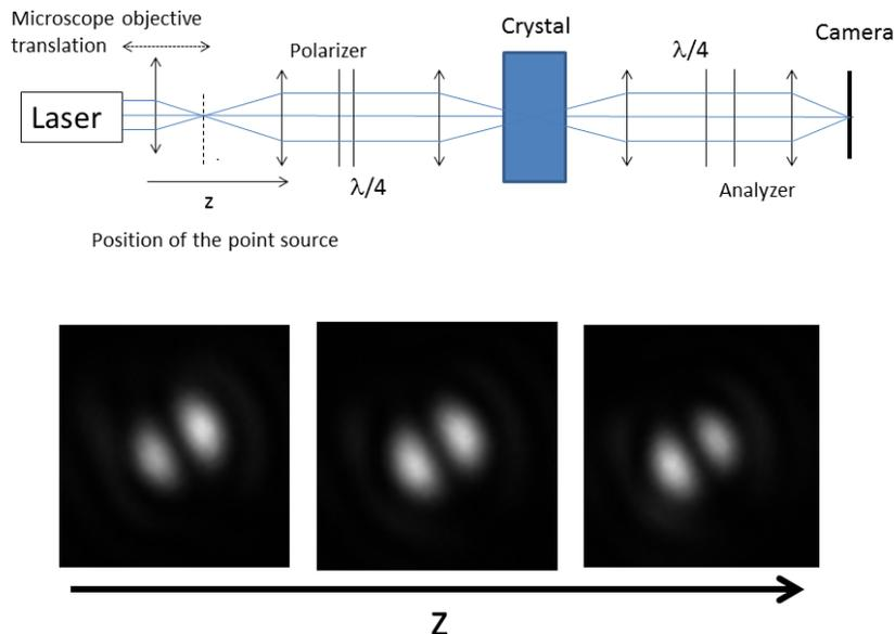
Figure 5. Top: Scheme of the set-up to observe Z-varying distributions. Bottom: images on the camera of the generated distributions for different values of  $z$
