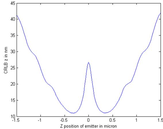
Figure 10.  $CRLB_z$  of a PSF shaped by conical diffraction with an ellipticity parameter of 10 degree and crystal thickness parameter of 1mm. This PSF is good for operating at a range of  $3\mu m$
