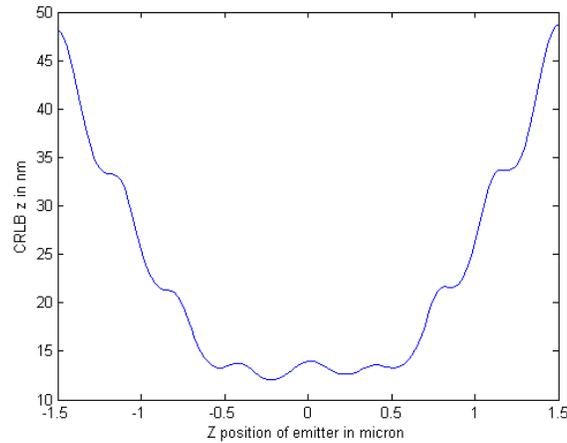
Figure 11.  $CRLB_z$  of a PSF shaped by conical diffraction with an ellipticity parameter of 20 degree and crystal thickness parameter of 0.8mm. This PSF is good for operating at a range of  $1\mu m$
